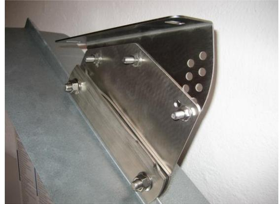
**Contents for one clamp holder:** 2 x brackets, 1 x mounting part, 1 x upper angle-part, 2 x screws M12 x 35, 2 x carriage nuts M12 (hexagon), 3 x screws M8 x 20, 3 x carriage nuts M8 (hexagon)
